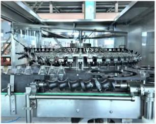
RINSING PART Neck Control with plastic snap on the gripper.
